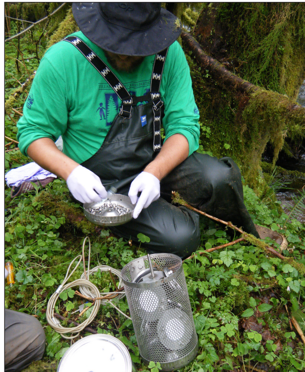
Above: TEP staff deploying POCIS device in the upper reaches of Fawcett Creek, one of Tillamook's drinking water source streams.
